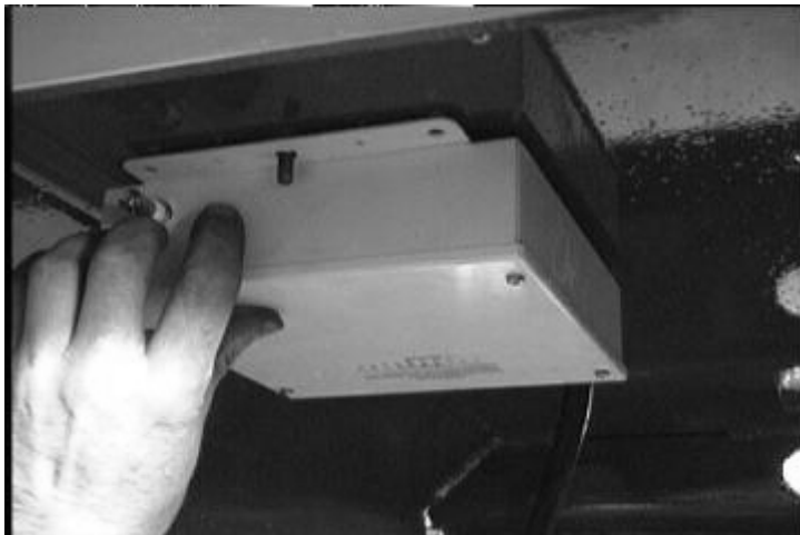
INSTALL REMOTE BOX IN TOP OF TOOL BOX
